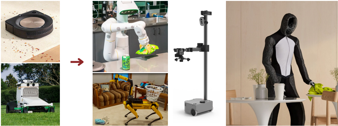
Figure 1.1: Household robots are evolving from task-specific machines, such as vacuum cleaners or lawn mowers (left), to general-purpose assistants capable of tackling a diverse array of tasks such as tidying up (right). Courtesy: (from left) iRobot , Scythe Robotics , Alphabet , Boston Dynamics , Hello Robot , 1X Technologies
