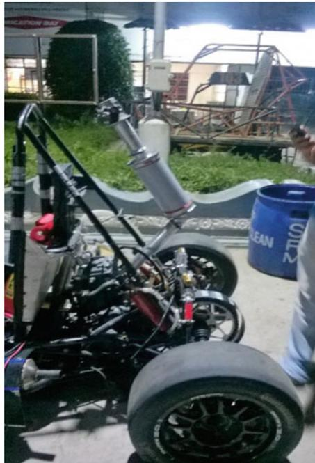
Fig. 5 PVC Intake iterative setup
