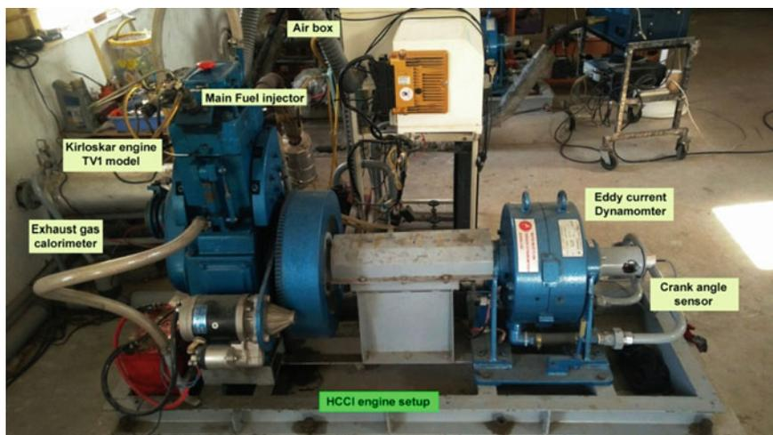
Fig. 7 Test engine setup
