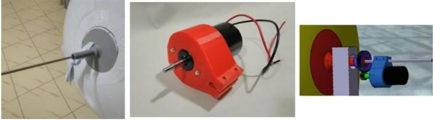
**Fig. 6** 3D printed pipe and the stainless-steel shaft mounted on the balloon, generator in its mount, CAD model for the translation mechanism
