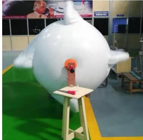
The shaft was divided into two parts which is mounted on both the sides forming a cantilever. To support this cantilever, we have provided 2 supports with ball bearings. The final mechanism was coupled with the balloon with the help of anabond adhesive and was very strong without any slippage between the balloon and the mechanism (Fig. 14).
