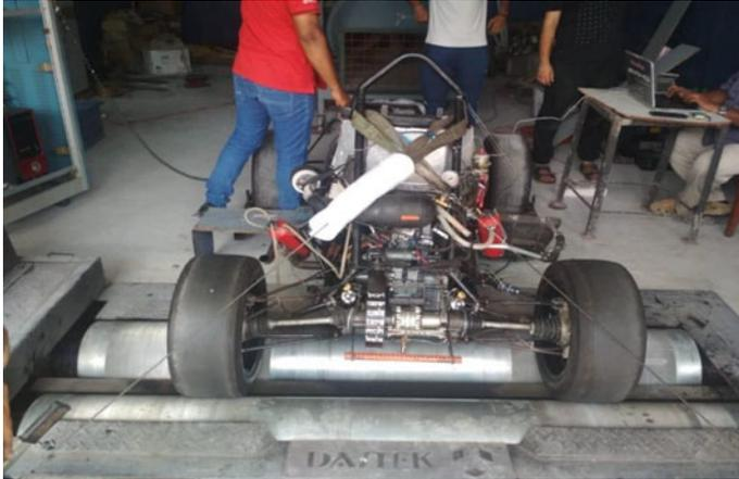
**Fig. 15** Commercial eddy current dynamometer
